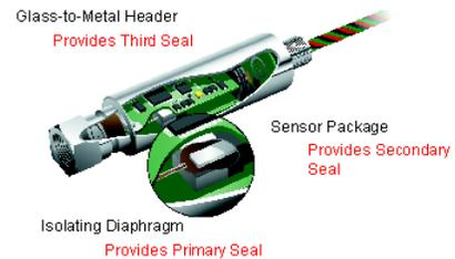
*The standard requires that devices provide two or more reliable seals capable of withstanding full process pressure at operating conditions or pass a series of severe tests to prove reliability.*
