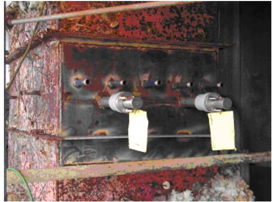
Primary elements and the traverse test points in the duct
