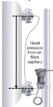
A change in process temperature induces the fill-fluid density to change within the capillary. This change in density causes a measurement shift due to the head pressure varying.
