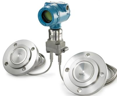
A balanced system has identical diaphragm seals and equal lengths of capillary on both the high and low side of the DP transmitter.
