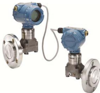
With a Rosemount 3051S ERS System, a digital signal replaces impulse lines and capillary to increase measurement reliability and performance on tall towers and vessels.
