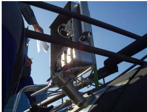
Figure 7: Stackbar installed in a stack with automatic purge system.
