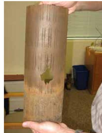
*Cut liners from over-injection of steam is one of the hazards of poor steam injection control*
