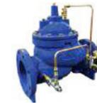
The pressure sustaining valve uses a solenoid override and anti-cavitation trim to open and dispense water from 100+psi to atmospheric pressures with a tunable flow.
