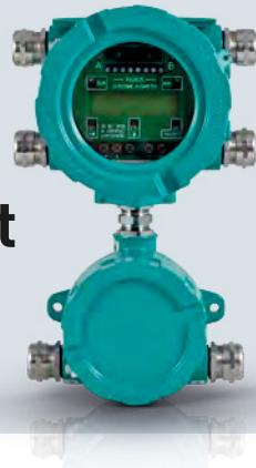
The WavelInjector® has been specifically engineered for high-temperature applications. Using patented technology, the WavelInjector® thermally separates ultrasonic transducers from the hot pipe, allowing operation at process temperatures up to 400 °C and beyond.
